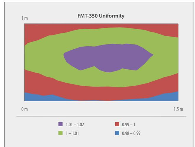
The uniformity of the FMT-350 is Class A ( $\pm 3\%$ ) over 1 m x 1.5 m.
