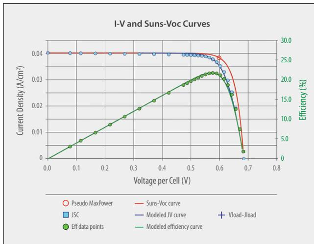
The FMT interface displays both I-V and Suns-Voc data. This permits direct comparisons of module data to cell data and quick identification of series resistance, shunting, and cell mismatch.
