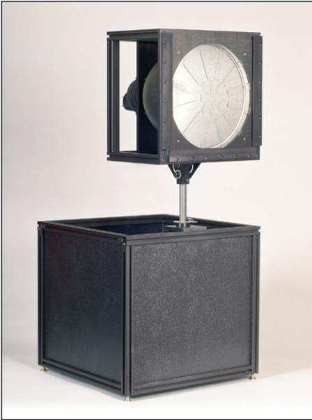
Advanced analysis of solar modules including light I-V and Suns-Voc data. Capability to accurately measure high-efficiency modules.
